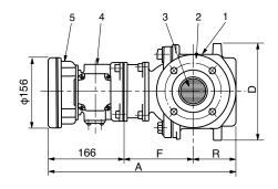
Transmission Gear Box w/External Accuracy Adjustor (GB2-0 15)
